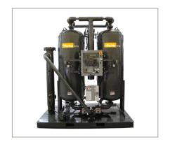
By "down flow" drying, the air exits the dryer at the bottom of the bed. Any condensation or liquids put into the dryer by ineffective pre-filtration or drain failure will collect at the bottom of the vessel. As a result of this liquid presence, with "up flow" regeneration the purge air cannot lift the liquid slugs through the entire desiccant bed resulting in liquid being sent down stream at tower switch over.
